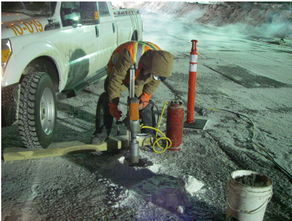
Photo 6: Collecting a core sample using the concrete coring machine. Photo looking east from around Sta.0+80.
